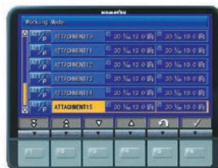
Komatsu Integrated Attachment Control (KIAC)
